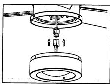
Securely attach 9-pin connector from motor assembly to wiring harness socke within light kit assembly.
