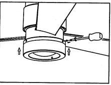
Assemble the light kit assembly onto the motor assembly using the previously removed screws.
