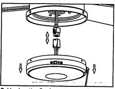
Unplug the 9-pin connector from motor assembly and switch cup housing.
