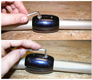
When the screws are securely fastened, the downrods should be sturdy and there should be no movement.
