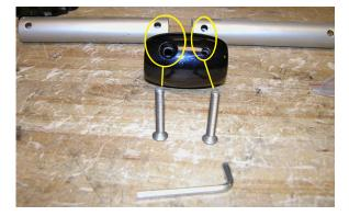
Insert the down rods into to each side of the coupler. Insert the screw into the larger tapered hole and run it through the downrod until you are able to securely tighten the screw into the threaded side of the coupler. Turn the coupler over and repeat on the other end.
